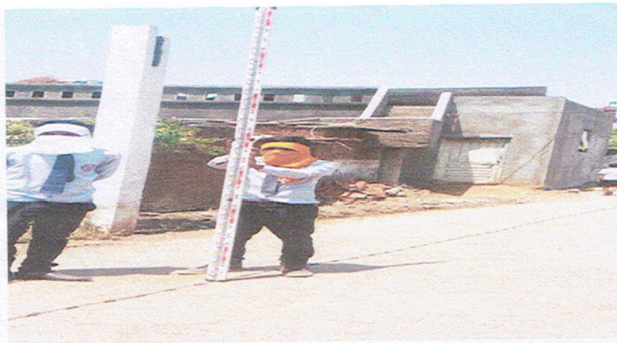
Image 4: Taking a reading on Bench Mark
